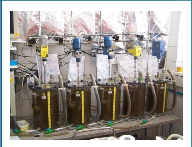
Fig. 2: Stirred tank reactors of the labscale biogas plant
