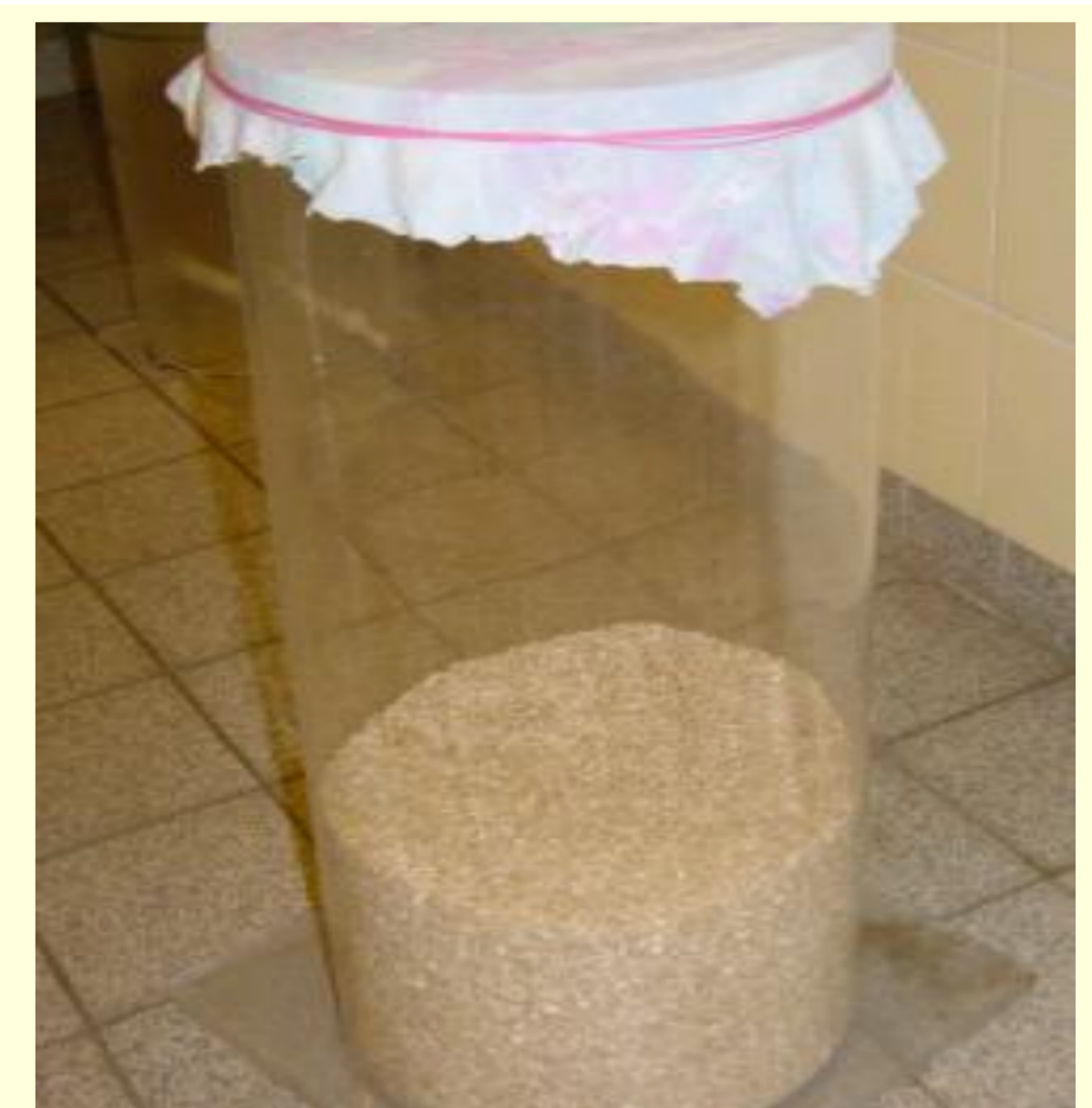
Fig. 2: A glass cylinders (50 cm height, Ø = 25 cm) with organic rice with a moisture content of 14%.
